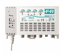
3-input (III+DAB, UHF, UHF) multiband TV indoor amplifier with 32dB gain and up to 120dBµV output level on UHF band, separate amplification with independent level adjustment (20dB) for each input and low noise figure. T2 technology with UHF cut band for LTE 4G @790MHz and 5G @694MHz.
