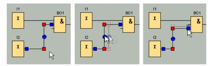
If you do not connect a line to a suitable target connector, LOGO!Soft Comfort reconnects it to its initial position after you "release" the mouse button.
