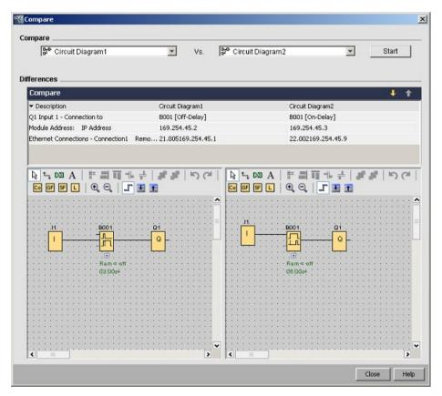
Result: As shown in the result display above, the two compared circuit programs have different module address settings and different IP address settings for two Base Modules that are both used as clients.
