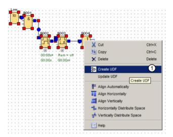
If the selection includes blocks that a UDF does not support, LOGO!Soft Comfort excludes them from the UDF. If an included function block is connected to an excluded one, LOGO!Soft Comfort creates an input or output in place of the excluded block. If the number of inputs and outputs would exceed the restrictions, LOGO!Soft Comfort does not make inputs or outputs that would exceed the restriction.
