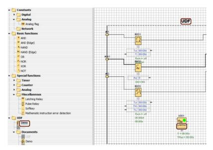
Double-click the UDF identifier above the expanded UDF to open the following properties dialog. You can enter up to eight characters for the UDF name. You can also password-protect the UDF in the following dialog:
