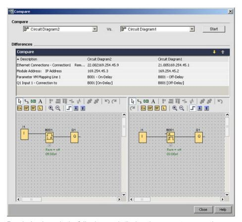
Result: As shown in the following result display, the parameter names in parameter VM mapping line 1 of the two circuit programs are different.
