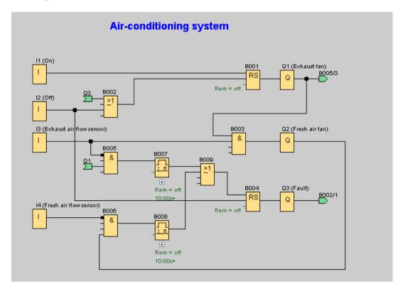
You can invert output Q3 to use output messages at Q4. Relay Q4 only drops out if main power is lost or if there is a fault in the system. The output can then be used for a remote message.
