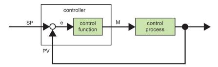
The comparing element and the controller function describe the conduct of the controller.
