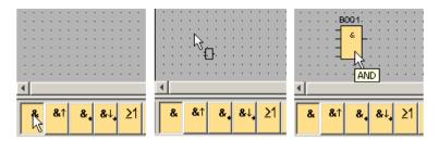
There is no need to align the blocks right away. A precise alignment of the blocks at this time does not make sense, until you have interconnected them and entered the comments in your circuit program.
