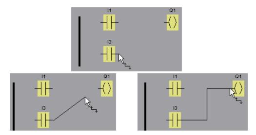
LOGO!Soft Comfort offers you a further option of connecting blocks when you right-click the input or output of a block. In the shortcut menu, click the **Connect with block** menu command to display a selection list that contains all blocks available for your connection. Click the relevant target block. LOGO!Soft Comfort then draws the connecting line. This method is especially useful for connecting a source to a target block over a greater distance on the programming interface.
