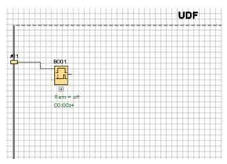
To remove an input/output, select the yellow connector figure and select "①" in the context menu. The corresponding connection line(s) will be deleted as well:
