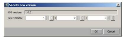
The new version must be an increment from the previous value. For example, in the example shown above, version 1.0.3 or 0.254.3 would be invalid.
