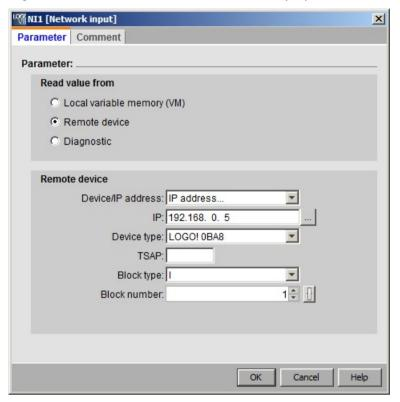
The configure items are different for different device type, for example you need to input the port and Unit ID for connecting a Modbus-compatible device.
