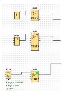
LOGO!Soft Comfort displays a warning signal (!) in the upper right corner to indicate that the UDF is out of date. You can right-click the block, and select "①" from the following context menu to update the UDF to a new version.
