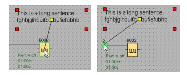
A linked comment moves consistently with the figure to which it is attached. You can adjust the relative position of the comment to the figure, as you do a block comment.
