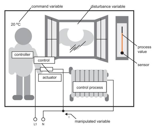
The control device consists of the actuator and the control.
