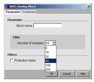
After you set the parameter, the analog filter calculates the average value of the samples and assigns this value to AQ.
