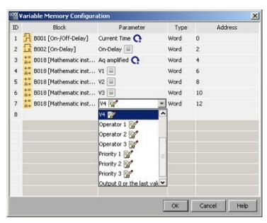
The Block column lists the parameters for SFBs in the current program. The Parameter column provides a select list of the parameters of the corresponding block. The Type column displays the data type of the selected parameter. The Address column is also configurable. You can use it to identify the VM address used to save a parameter value.
