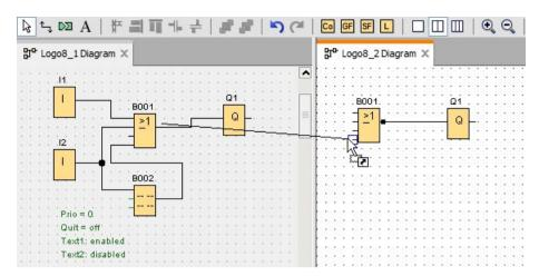
When you connect two function blocks in two separate circuit diagrams, LOGO!Soft Comfort creates a pair of network function blocks, including the Ethernet connection and data transfer mechanism. The green color indicates that the LOGO! device of the two circuits are connected in LOGO!Soft Comfort. The network function block turns to red if its LOGO! device loses the connection to the other LOGO! device in LOGO!Soft Comfort.
