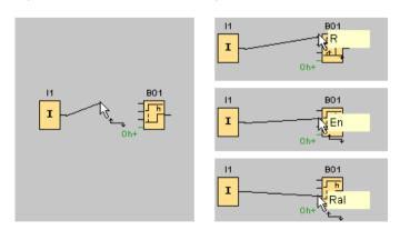
LOGO!Soft Comfort displays a blue frame around the mouse pointer when it can connect to an block input (pin)
