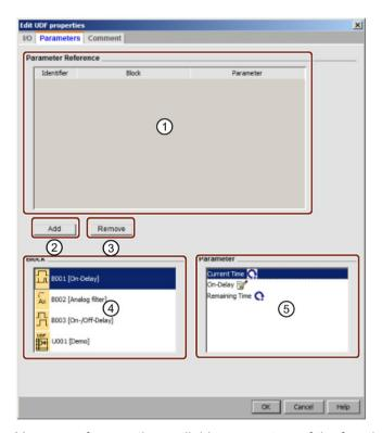
You can reference the available parameters of the function blocks used in the UDF as the parameters of the UDF. "④" shows the function blocks, while "⑤" shows the parameters that the selected block includes. Double-click a parameter or use "②" to move a parameter from "⑤" to "①".
