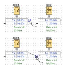
The reference line between two parameters indicates their reference relation. You can delete the reference line to remove the reference.
