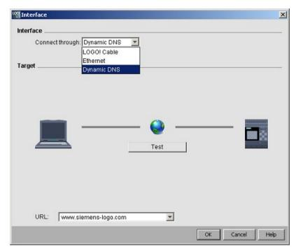
You must configure your router in order to access the LOGO! Base Module through dynamic DNS. Make sure you have completed the following settings before connection:
