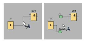
The connection is closed again by clicking on its open end while the Cut/Join tool is active. Optionally, you can close the connection by right-clicking on an open end and calling the **Join** menu command.
