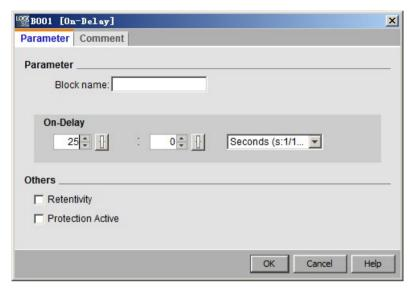
The block properties dialog box consists of several tabs. Every block has a Comment tab, where you can enter relevant block comments. For some blocks a Parameter tab is available where you can describe specific block parameters. You configure input simulation parameters from the Simulation tab.
