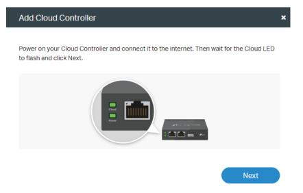
4) Click **Next** to load the following page. Enter the device key, which is displayed on the back of the Omada Cloud Controller. Type the characters in the Image.
