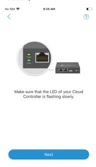
4) Click **Next**. To bind the Omada Cloud Controller to your TP-Link ID, you can either scan the QR Code, or enter the device key manually. The QR Code and device key are displayed on the back of the Omada Cloud Controller.
