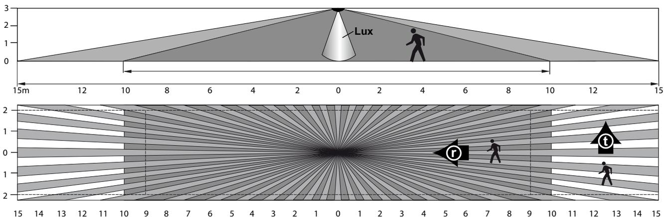
The detection range in side view (top) and top view (bottom).
