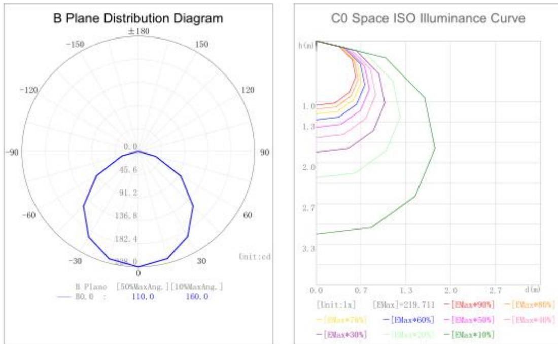
● Lux test diagram
