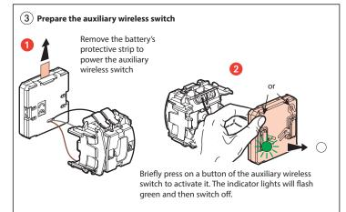
Do not install the auxiliary wireless swich in its box. The installation will be completed in steps 6 & 7.
