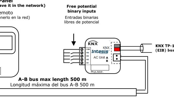
**NOTE:** In some indoor unit models the A-B is not available. In its place there is a pair of cables to connect the Control Panel. Use these cables to connect the A-B bus. Check your indoor unit user or service manual for more information.
