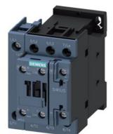
Contactor, AC-1, 35 A/400 V/40  $^\circ\text{C},$  S0, 4-pole, 230 V AC/50 Hz, 1 NO+1 NC, screw terminal
