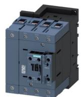
Contactor, AC-1, 160 A/400 V/40  $^\circ\text{C},$  S3, 4-pole, 230 V AC/50 Hz, 1 NO+1 NC, screw terminal
