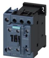
contactor AC-1, 50 A, 400 V / 40 °C, 4-pole, 230 V AC, 50 Hz, auxiliary contacts: 1 NO + 1 NC, screw terminal
