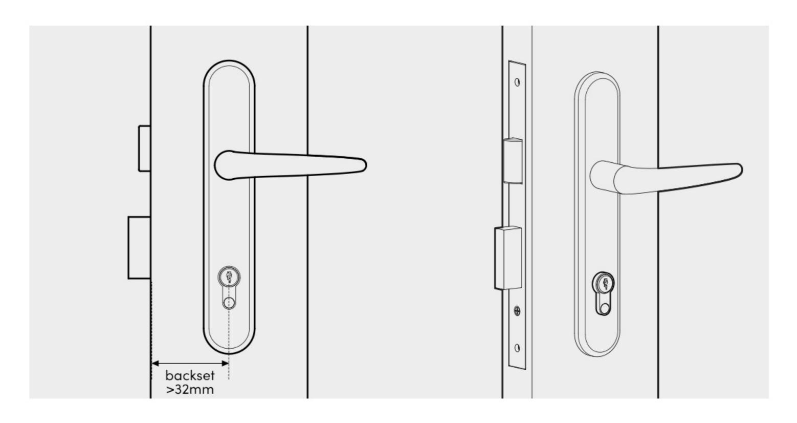
Distance from the euro cylinder to the edge of the door >32mm
