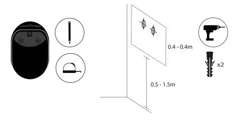
Fix the device to the wall by tightening the screws.
