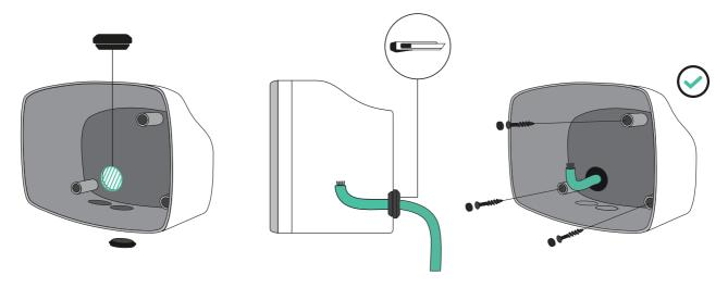
Fix the charger on the wall using the appropriate screws.
