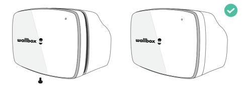
• Recommended tightening torque 0.7 Nm +/- 10%
